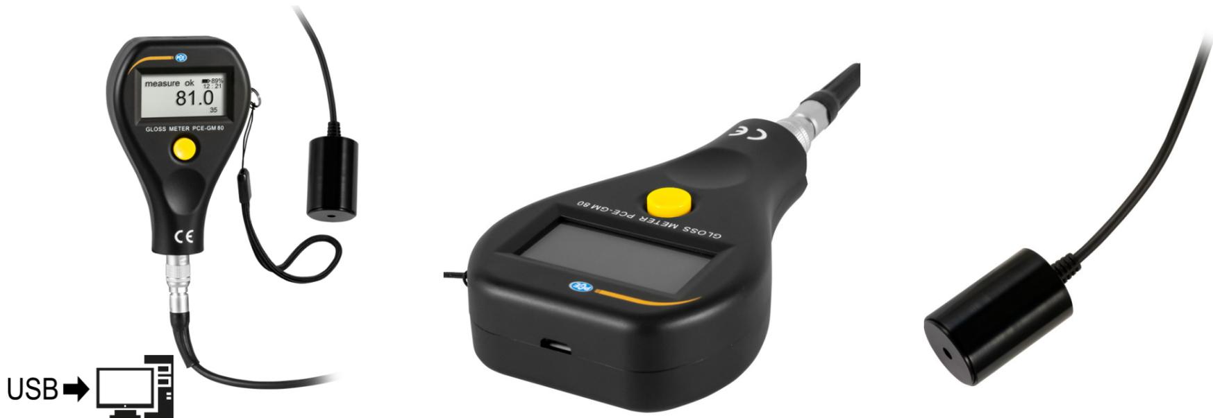
**Gloss meter with external gloss sensor / Measurement geometry 60° / Measuring surface Ø4.5 mm**
