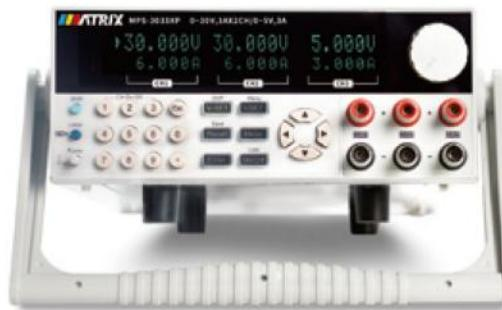
Triple channel programmable DC power supply is with high resolution, high precision and high stability. Over-voltage and over-heat protection are available. Series and parallel operation are also provided. The resolution is 1 mV / 1 mA.
