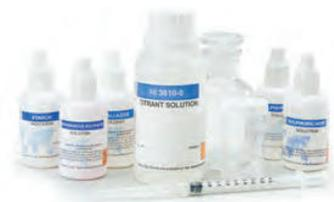
The HI3810 is a titration-based chemical test kit that determines the dissolved oxygen concentration within the 0 to 10 mg/L  $\text{O}_2$  range. The HI3810 is supplied with all of the necessary reagents and equipment to perform the analysis. The test kit contains enough reagents to perform approximately 110 tests.
