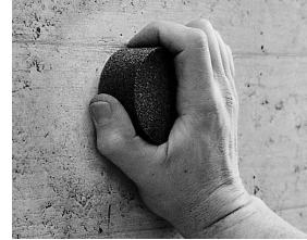
Fig. 2.1 Preparing the test surface
