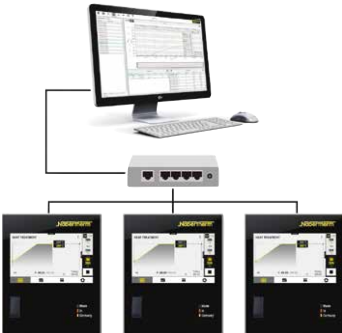
Example lay-out with 3 furnaces
