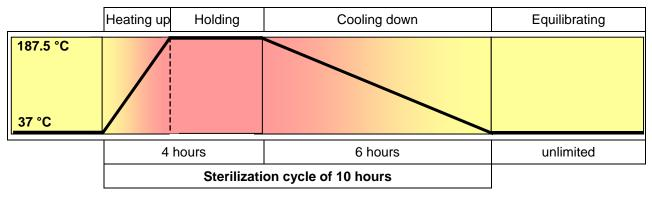
Figure 33: Setpoint profile during the sterilization cycle
