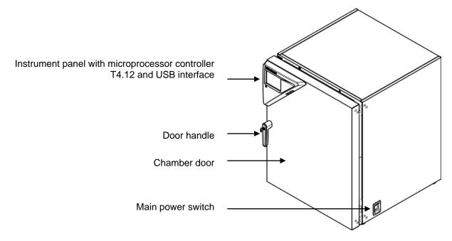
Figure 4: CO<sub>2</sub> incubator CB / CB-UL (example: model CB 170)
