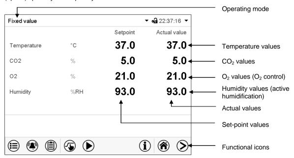
Figure 19: Normal display of the MB2 program controller (sample values, chamber with  $O_2$  control and active humidification)
