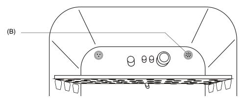
Figure 30: Position of the access port for extra-low voltage
