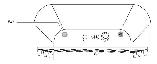
Figure 26: Position of the interior socket 230 V
