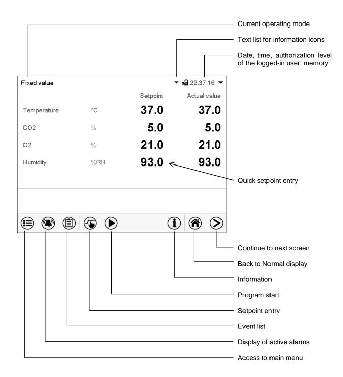
Figure 20: Operating functions of the MB2 controller in normal display (sample values, chamber with  $O_2$  control)
