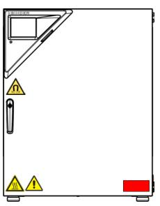
Figure 1: Position of labels on the chamber
