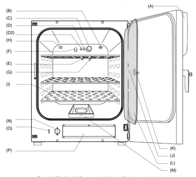
Figure 5: CB 170 with O<sub>2</sub> control, active humidification, and options
