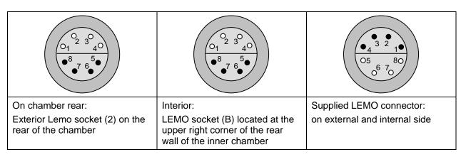
Figure 31: Pin allocation (front view) of the Lemo sockets and plug
