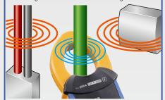
Minuscule leakage currents can be accurately detected since the meter is resistant to the effects of external magnetic fields.
