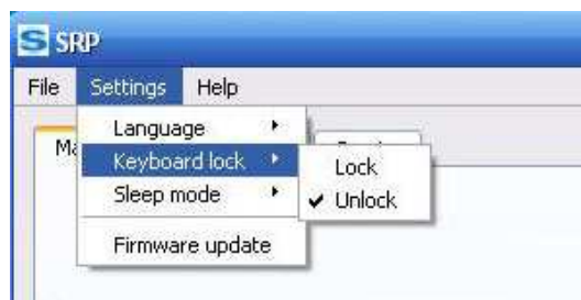
Figure 10 Locking the keypad.
