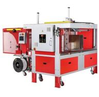
**TP-702CQ** is built based on TP-702C high speed corrugated strapper combined with the 4-side squaring station C1-BQ. It carries all the innovative features of TP-702C. The backstop, pusher, and side squaring altogether provide the precise bundle control and assure the bundle integrity during the strapping cycle. Easy bundle size change setup eliminates the downtime and makes the production more efficient. Truly user friendly machine for your Casemaking and Flexo Folder Gluer line.
