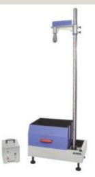
JIS-(K5400)、K5600-5-3、(K6718)、(K6745)、K7211、ISO-6272 This tester is used to evaluate the impact resistance of rigid plastic, coating
