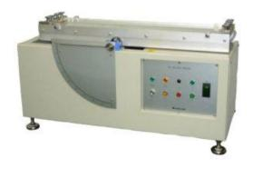
This tester is used to measure the Inclination Angle(Static Friction Coefficient) when the test specimen of enabled wire starts sliding.
