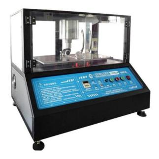
This instrument is mainly used to simulate the caster of the office seat repeatedly crushed on the wire to detect the crushing ability of the DC wire against the office chair wheel. This instrument is designed in accordance with the APPLE 080-1276-K standard.
