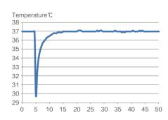
Temperature recovery curve (door open for 30s)
