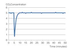
Co<sub>2</sub> concentration recovery curve (door open for 30s)
