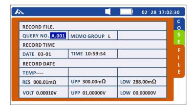
2. Use the key ( ) to select the memory number to be read out. Use the key ( ) to locate the memory number The measurement values for the selected memory number are displayed.
