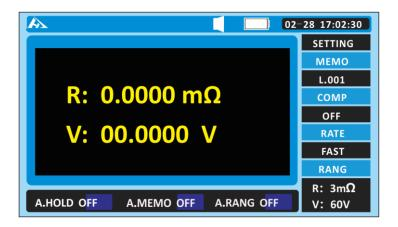
1. Press [SYS] on the test page. Switch to the comparator interface.
