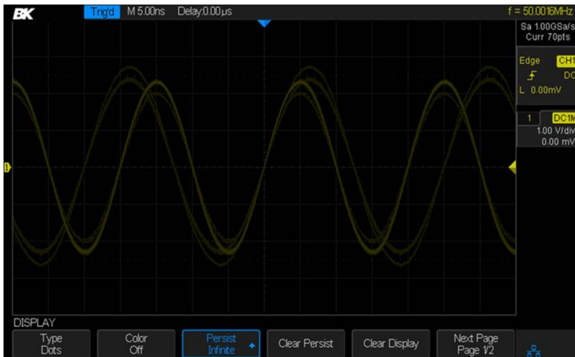
Figure 92 - Persistence set to infinite
