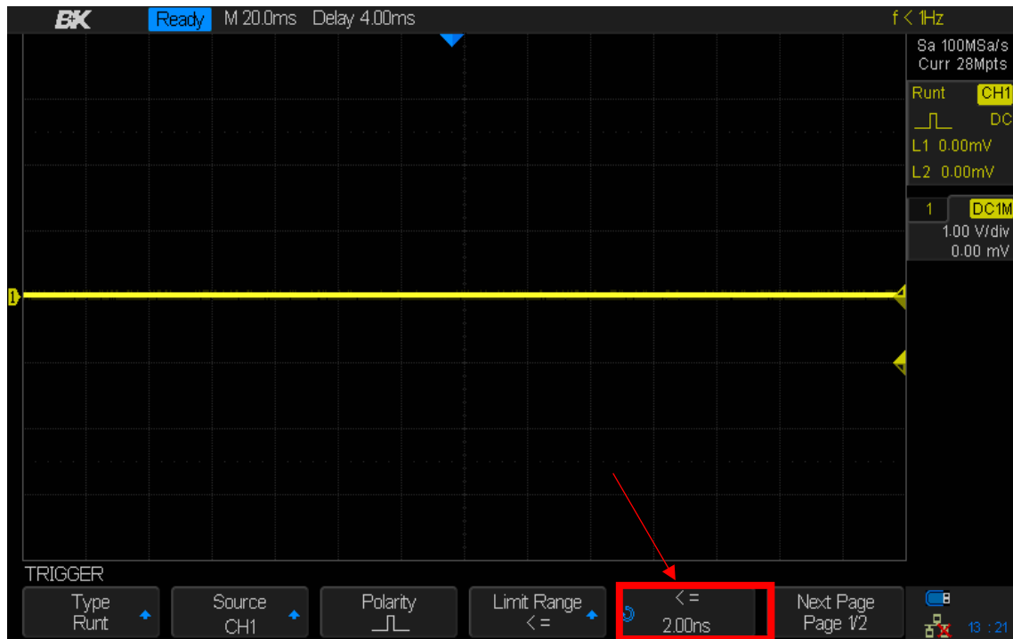
Figure 65 - Time setting runt trigger
