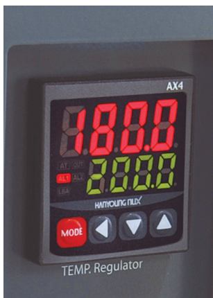
Individual over temperature limiter
