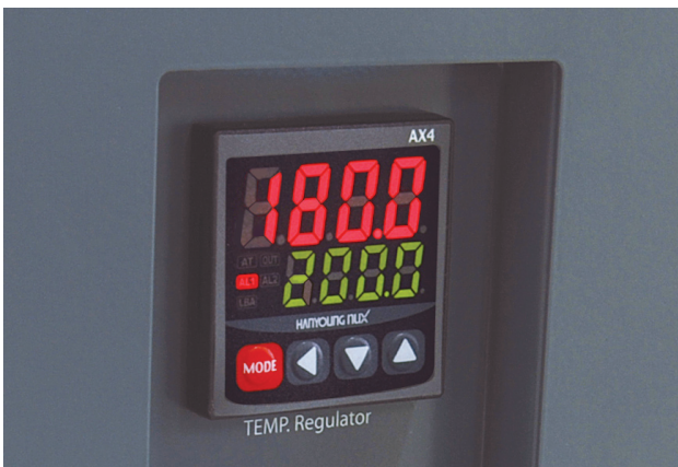
Individual over temperature limiter
