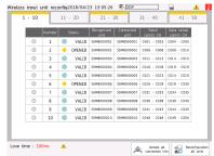
Wireless input unit reconfiguration display
