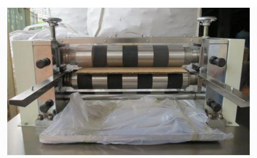
BATTERY ELECTRODE SLITTING PROCESS
