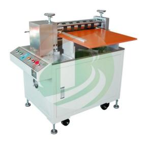
Lithium Battery Electrode Slitting Machine
