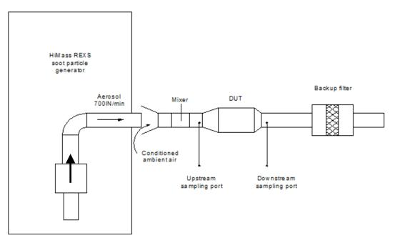
Fig. 6.4: The DUT is not directly connected to the aerosol output. In this measuring configuration the aerosol flow is diluted by conditioned ambient air
