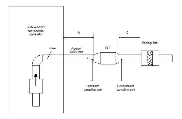
Fig. 6.1: Direct connection of the testo REXS to the DUT
