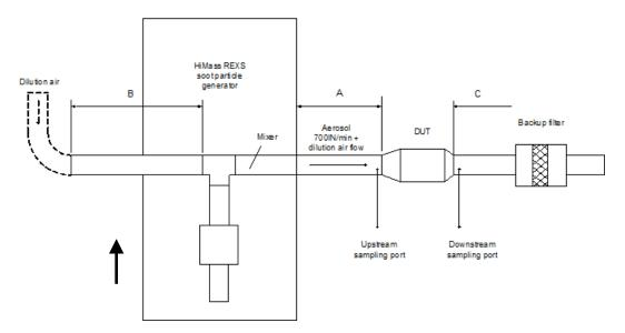
Fig. 6.2: Direct connection of the testo REXS to the DUT with additional dilution air supply
