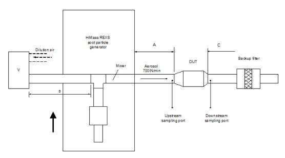
Fig. 6.3: Direct connection of the testo REXS to the DUT with additional dilution air supply with volume (V) to avoid pulsation
