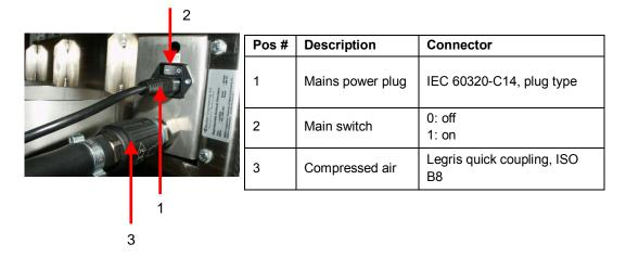
Fig. 4.8: Electrical and air connectors
