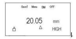
WHEN PROBE AND TEST SPECIMEN COUPLANT IS GOOD, THE DISPLAY WILL SHOW COUPLANT GOOD INDICATOR. WHEN LIFT-OFF THE PROBE THE THICKNESS DISPLAY NO CHANGE BUT COUPLANT INDICTOR DISAPPEAR.
