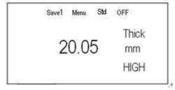
USE KEY TO ADJUST THE THICK THICKNESS DISPLAY UNTIL MEET BLCOK THICKNESS VALUE. THEN PRESS CAL KEY AGAIN. COMPLETE THE 2-PINT CALIBRATION SETUP.
