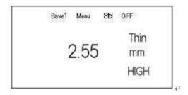
USE KEY TO ADJUST THE THIN THICKNESS DISPLAY UNTIL MEET BLCOK THICKNESS VALUE. THEN PRESS CAL KEY AGAIN. DISPLAY
