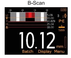
The B-Scan vertical scale can either be set to 'Auto' or the user can set the scale most appropriate for the thickness of the material under test.
