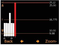
Subsequent presses of the ← softkey will scroll backwards, pressing the → softkey will scroll forwards through the readings, 25 readings at a time.
