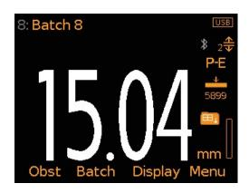
Note: The number of readings within the batch includes those recorded as 'Obst' however, 'Obst' readings are not included in statistics calculations.
