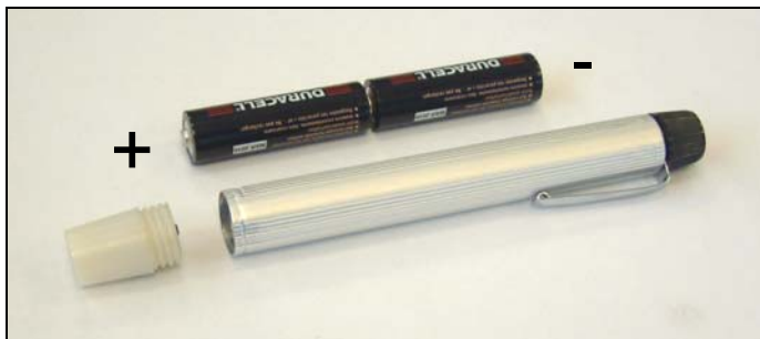
Figure 1. Microscope light source - battery polarity
