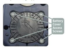
Replace all batteries at the same time. Ensure on replacing the battery cover that the gasket is correctly located to prevent any water ingress. Tighten the screws carefully but do not overtighten.
