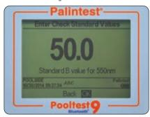
Use the up/down keys to adjust the values to match the certificate, following the order defined on the display. Press OK when the correct value is shown and the prompt will forward to the next value.
