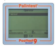
Choose the Operator ID to be used by scrolling through the list and pressing the OK key on the desired choice. The instrument will return to the System menu.
