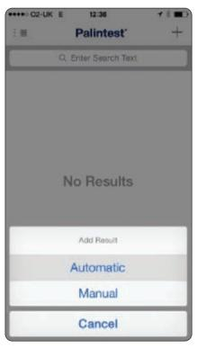
To connect the Pooltest 9 Bluetooth press the '+' symbol in the top right hand corner of the device screen. This will produce the list of all locally advertising Bluetooth SMART devices.
