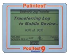
If the connection is lost the Pooltest 9 Bluetooth will prompt for re-connection. If connection is not required or possible press Exit to disable Bluetooth and cancel the log transfer.
