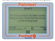
Ensure the blank cuvette is being used, not the sample plus reagent cuvette. Sample colour can be reduced by dilution with clean water; the dilution selected should take account of the expected concentration of parameter under test. Blank results are stored in the temporary memory of the Pooltest 9 Bluetooth and will be used for all subsequent tests until:
