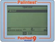
To create a new Operator ID, select Operator ID and use the up/down keys to select a blank field. Select New and press OK.
