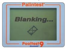
The Pooltest 9 Bluetooth will determine the absorbance due to the sample colour at all wavelengths simultaneously and store in temporary memory for use in analysis.
