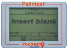
Insert the Blank cuvette and press OK.
