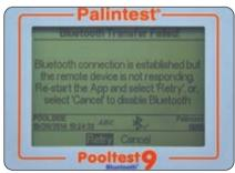
The Pooltest 9 Bluetooth is not receiving a response from the Palintest Aqua Pal app but the remote device is connected. This will appear 10s after a result transmission has started and no valid response has been received.
