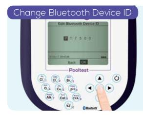
To change the Bluetooth Device ID, Select 'Bluetooth Device ID' and change as required.
