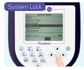
The system settings can be locked to prevent changes. From the main menu, select 'System Mode', then 'System Lock'. To lock or unlock the instrument enter the code 6812. To change this code, contact Palintest.
