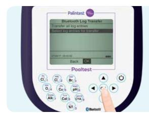
To transfer a specific log file, highlight 'Select log entries for transfer'. Use the up and down arrows to find the correct log entry and select OK. 'Log transfer complete' will display when the process is complete
