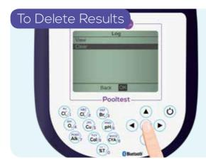
To delete results from the log, select 'Clear', this will permanently remove all results from the log. Operator IDs and Sample IDs will be stored in the results log to show which operator performed the test and which sample was used.
