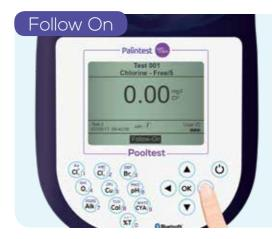
Refer to the test method to see if this is required. If a follow-on test is available, it will appear in the bottom menu. Select if required.
