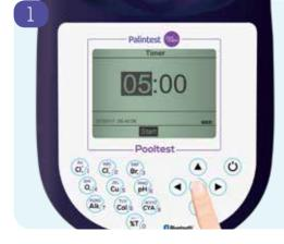
A timer can be set after the blanking process. Refer to the test method to see if this is required. The development time for the test will automatically appear. This can be modified using the arrow keys. Press start to set timer running.
