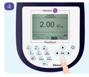
When the test is complete, the result will display on screen.
