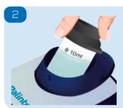
Insert the tube with the orientation mark ◊ facing forward and press read. An audible tone will sound after each reading.
