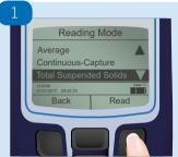
This mode will only be active if a site calibration has been stored within the Turbimeter. Once a calibration has been created, the Sample ID can be used to recall the site specific relationship between turbidity and suspended solids.
