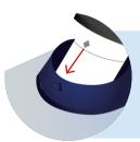
Place the sample tube in the instrument in the same orientation for all readings.
