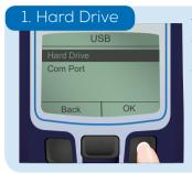
To download results and calibration logs, or to update the instrument firmware the device must be in 'Hard Drive' mode.
