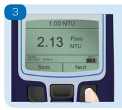
'Pass' will appear onscreen if the result is within the tolerance displayed on the standard. If the result is outside of the tolerance, the instrument may need to be re-calibrated. For field use, a set of SDVB (styrene divinylebenzene) calibration standards are provided to check the factory calibration and recalibrate the meter if necessary. Only SDVB standards from Palintest can be used with the Turbimeter Plus.
