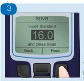
The instrument will request the remaining standards in order of increasing turbidity value. After the final standard has been read, the screen will show a countdown timer. When the calibration process is complete the screen will show
