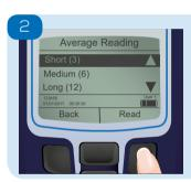
Select the number of readings required: Short (3), Medium (6), Long (12). Insert the sample with the orientation mark  $\Diamond$  facing forward and press 'Read'.
