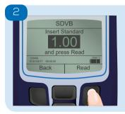
Use the Up/Down buttons to adjust the value on screen to that on the standard and press 'Read'.
