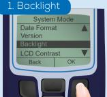
The instrument display features a high intensity backlight for use in low light conditions.
