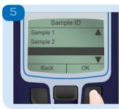
To record results without a Sample ID. Select a blank entry by scrolling to the bottom of the list and select 'Back'.
