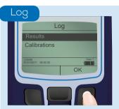
From the main menu select 'System mode' then 'Log' where the 'Results' and 'Calibrations' logs are stored. In both sections there is a choice to either view or clear data.
