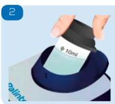
Select the Sample ID for the site/sample. The calibration data will be recalled automatically. Insert the sample with the orientation mark  $\Diamond$  facing forward and press 'Read'.
