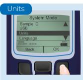
To change units which results are shown in, from the home screen press 'System' mode then 'Units'.
