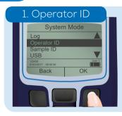
To access operator ID from the home screen press 'System' mode then 'Operator ID'. Up to 12 Operator IDs can be created. When selected, the ID will appear in the info panel on screen as well as in the log.
