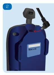
Once the device is in 'Hard Drive' mode connect to a PC, using the supplied USB cable.
