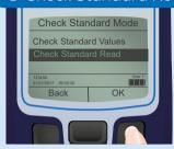
Select the Check Standard Read option to perform a recorded read back of each turbidity check standard.
