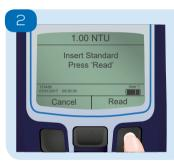
Follow the on-screen prompts and insert the Check Standards as requested. Select the Read button to perform the measurement.
