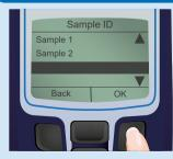
Highlight the ID and select 'OK'. The screen shows the option to select either 'Edit' to change the ID, or 'Delete'. Deleting the sample ID will not affect results stored in the log.
