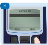
To create a new Sample ID Scroll to the bottom of the list, then select 'New'. Use the Up/Down buttons to select characters. When the correct character is shown, press and hold the [+] key to move to the next
