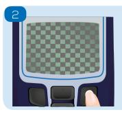
The LCD screen contrast can be manually adjusted. Use the up/down buttons to adjust the contrast until the alternating shapes are clearly visible and press 'Save'.
