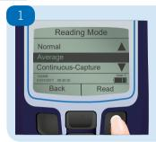
This mode takes multiple measurements and averages the results. Three options are available: Short (3 readings), Medium (6 readings) and Long (12 readings).
