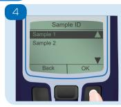
Select 'OK' on the Sample ID to be used. When selected, the ID will appear in the information panel on screen as well as in the log when results are stored.
