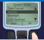
From the main menu select 'Sytem mode' then 'Version'. The serial number of the instrument and the software version are displayed.
