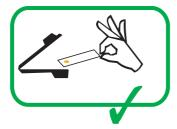
When removing filter paper from slide one should only observe a perfectly symmetrical colour stain, i.e yellow circle. If yellow stain goes beyond circle this suggests a gas leak which will give a low result. Repeat test ensuring Black Filter Slide is closed properly to maintain gas tight seal.
