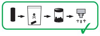
If internal cotton wool turns black within the Hydrogen Sulphide Removal Filter, DISCARD in waste bag and insert NEW FILTER.
