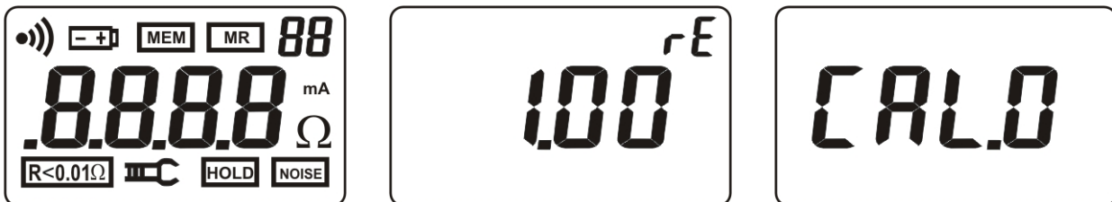
Fig. 2: Sequence of screens upon switching on the instrument
