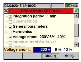
Fig. 75: Voltage Anomalies screen - setting control parameters
