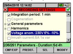
Fig. 74: Voltage Anomalies selection screen
