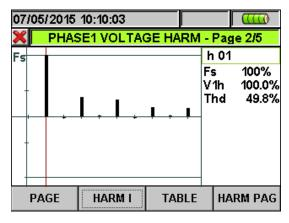
Fig. 37: Harmonic analysis voltage V1 in percentage values for 4-wire system
