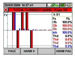
Fig. 117: Total harmonics in three-phase 4-wire system
