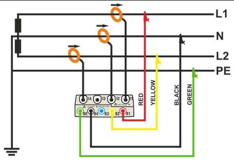
Fig. 147: Meter connection in a two phase 3-wire 1PH3W system - ENG\_UK type
