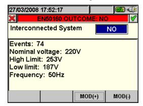
Fig. 110: Parameters set for EN50160 analysis
