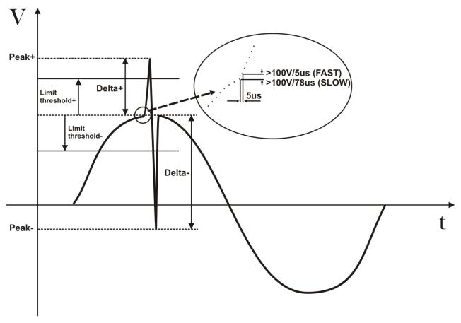
Fig. 151: Typical voltage spikes at 50Hz frequency
