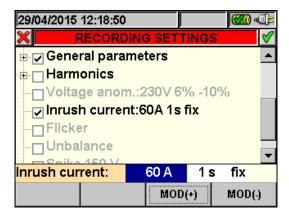
Fig. 77: Inrush current screen - setting control parameters
