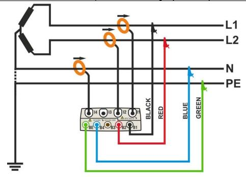
Fig. 142: Meter connection in a two phase 3-wire 3P2E system – ENG type
