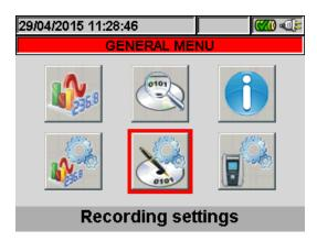
Fig. 63: Recording Settings screen selection
