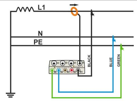
Fig. 130: Meter connection in a SINGLE phase system
