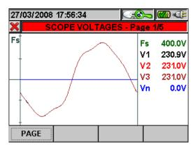
Fig. 116: Voltage scope in three-phase 4-wire system
