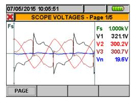
Fig. 28: Voltage waveforms screen for 4-wire systems
