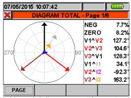
Fig. 39: Vectorial diagram total for 4-wire system
