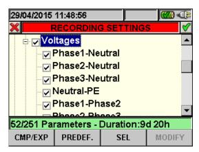
Fig. 69: General Parameters sub-level – Three phase 4-wire system
