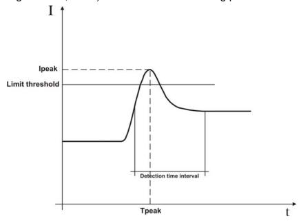
Fig. 148: Parameters of standard inrush current event
