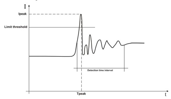
Fig. 149: Parameters of oscillating inrush current event
