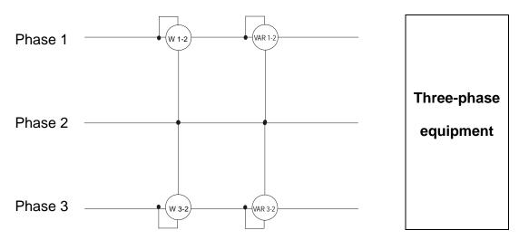
In this case the potential of one of the three phases (for example, phase 2) is taken on as reference potential. The total values of the active, reactive and apparent power are expressed as sum of the indications of the couples of Wattmeters, VARmeters and VAmeters.
