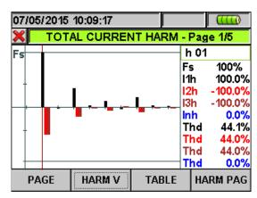
Fig. 34: Harmonic analysis of currents percentage/absolute for 4-wire systems
