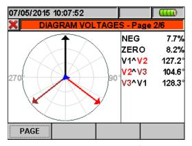
Fig. 40: Vectorial voltage diagram for 4-wire system
