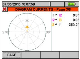
Fig. 41: Vectorial current diagram for 4-wire system
