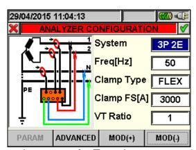
Fig. 54: Analyzer Configuration screen for Two phase system 3-wire 3P 2E - ENG type
