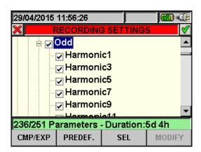
Fig. 71: Harmonics sub-levels: odd harmonics selection
