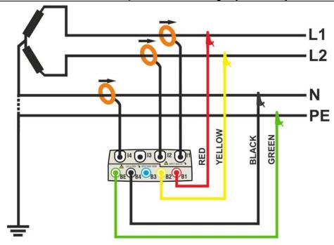
Fig. 143: Meter connection in a two phase 3-wire 3P2E system – ENG\_UK type
