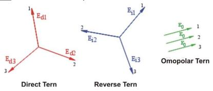
Fig. 150: Decomposition of a vectors tern
