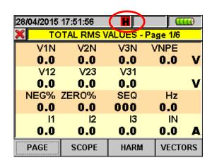
Fig. 4: HOLD function active at display
