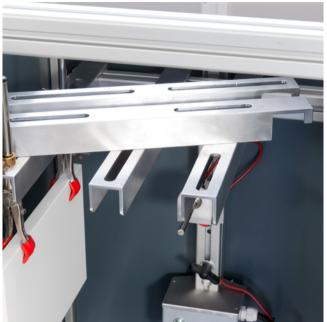
Test Cabinet for Damp Tests / based on AMK-MB-005 / automatic test sequence/ for up to 5 test pieces
