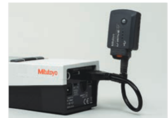
Example of the connection with SJ-210
