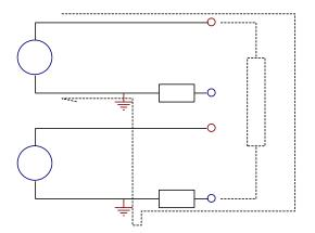
Because one point in the test low end of each unit structure is connected to the ground. Current is collected between the low end of the test and ground. The current loop of the high voltage of adjacent units can be achieved through the low end of the other units. The effect of this current on the measurement is as follows:
