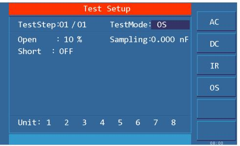
Figure 4.3.4 OS setting interface Open short circuit detection (OS) test parameters are as follows
