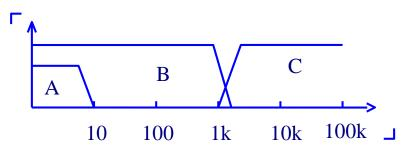
Comparison of frequency response of current overrun judgment and arc detection: (See the picture
