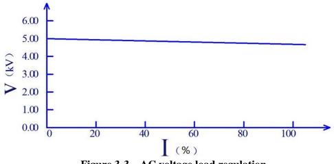
Figure 3-3 AC voltage load regulation
