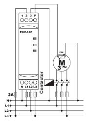
switched on and led switches off. In this case contact out is (NC)1 pole. PTC type phase failure relays are sensitive to thermal changes of motor. If the motor temperature is higher than optimum, relay releases, led switches off, when motor temperature is back to nominal, relay pulls and led switches on, relay releases when PTC resistance value 1600R-2000R and pulls again when resistance value 1000R-1400R.
