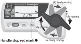
6 Press the "MEA." button, the decimal point blinks, the backlight lights up, the moisture content and measuring number are displayed thereafter. The backlight goes out after 4 seconds, but the moisture content remains being displayed.
