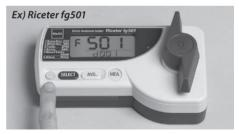
The backlight turns off and "Application", "Times" "%" are displayed. It is ready for measurement.
