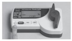
Press the "SELECT" button and repeat until the Selection Indicator and the abbreviation for name of application you wish to test appears. The selected application is memorized even after turning off the power.
