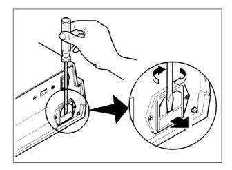
(3) Remove the fuses from the fuse holder and check to see if any are burned out.
