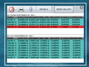
Automatic cycling and generation of the calibration report on a direct connected USB printer or generation of a PDF file. You don't need an extra computer and software to generate the report or to do the cycling!
