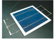
The 6-inch polycrystalline silicon cell of the test module is laminated, as a unit cell module, with white tempered glass, ethylene vinyl acetate (sealing material), and back sheet.
