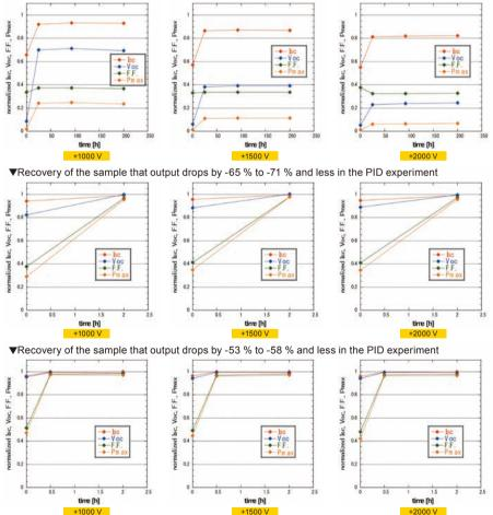
In the PID effect after conducting the reversible effect test, it may be found that the deterioration is reduced or recover nearly to the initial state in some module by being left or the reverse voltage is being applied. The polarity can be easily changed in TOS7210S with the switch.
