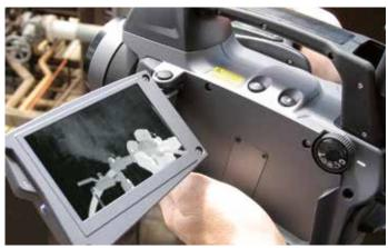
Tiltable, flip-out  $4.3^{\prime\prime}$  High Contrast Color LCD allows you to view targets more safely from any angle.
