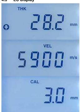
THK (thickness): material thickness measurement
