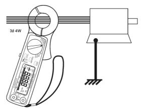
a. Set the rotary switch at desired range
