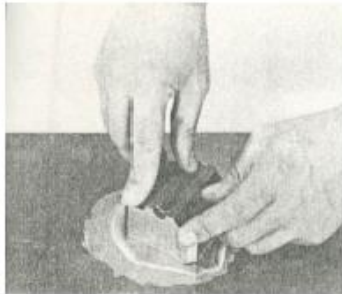
Mutual rubbing of both parts while firmly press the sample against the base plate.
