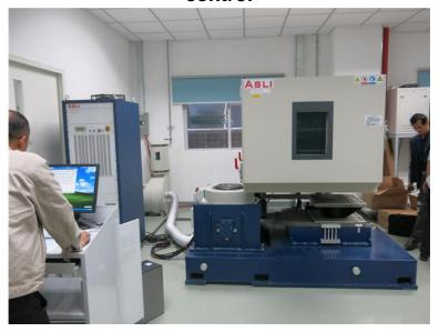
THV-1000-E Vibration Test chamber with temperature and climatic control
