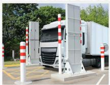
These types of detectors are widely used for the detection of radioactive materials that may be illicitly trafficked or unintentionally moved across international land borders, sea ports, airports, and similar locations, as well as at recycling plants or controlled access facilities. Fixed and deployable installed monitors are intended for radiation monitoring of vehicles, pedestrians and cargos. The networking capability allows for collecting and transferring data to a remote control center.
