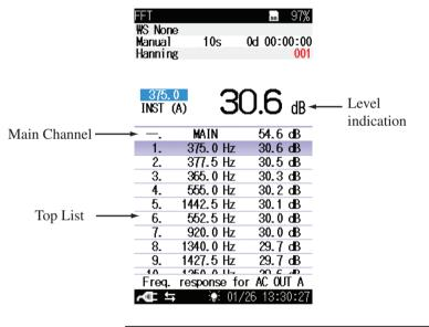
Note Pressing the MENU/ENTER key while MAIN is selected shows the main channel. Pressing the MENU/ENTER key while Top List is selected shows a bar graph for the frequency under the cursor. "--.-" is shown when the indicated value is -10 dB
