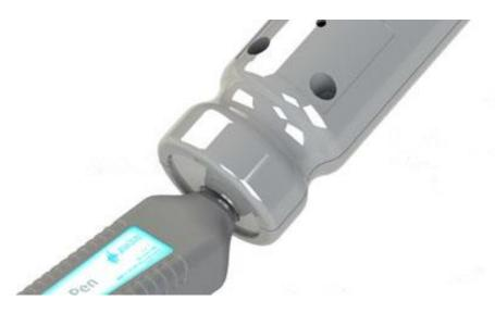
The calibrator should be the correct level for the configuration of the NoisePen, typically 94 or 114dB. Switch the calibrator on and press '**Calibrate**' in AnalyzerPlus. The result of the calibration will be reported, along with the present offset from the last factory calibration.
