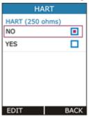
Select YES to add a Series resistor (250Ω) into the mA circuit. You can then use this instrument together with a HART® communicator to set up and calibrate HART® devices.
