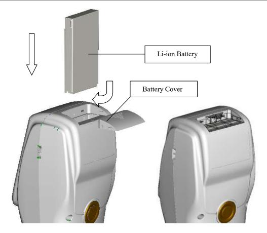
Figure 2 Battery Installation
