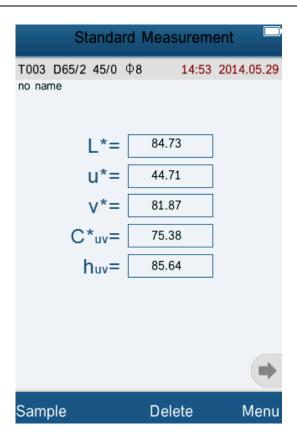
Figure 24 CIE L\*U\*V\* Standard Measurement
