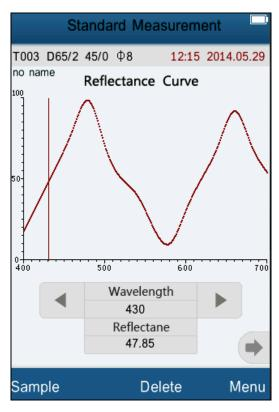
Figure 8 Spectral Reflectance Interface
