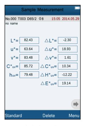
Figure 27 CIE L\*U\*V\* Sample Measurement
