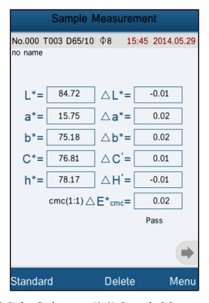
Figure 36 Color Index cmc(1:1) Sample Measurement
