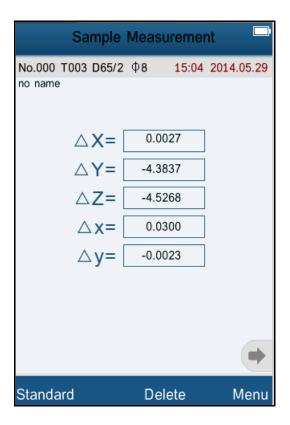
Figure 26 CIE XYZ Sample Measurement
