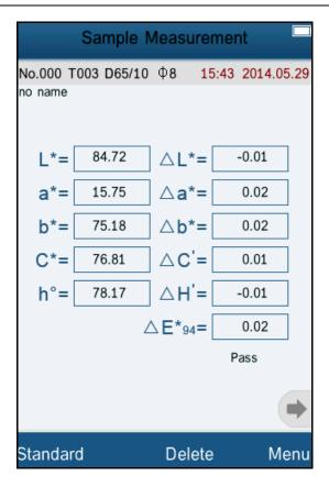
Figure 33 Color Index CIE94 Sample Measurement
