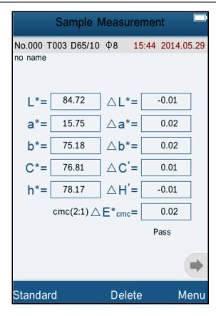
Figure 35 Color Index cmc(2:1) Sample Measurement
