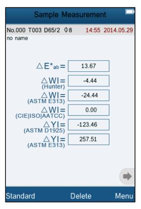
Figure 28 LAB &WI &YI Sample Measurement
