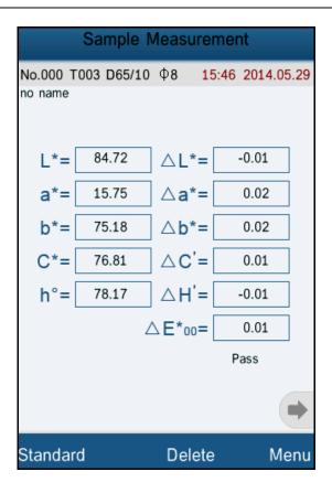
Figure 37 Color Index CIE2000 Sample Measurement
