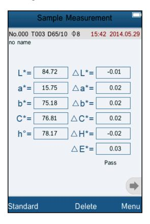
Figure 32 Color Index CIE1976 Sample Measurement
