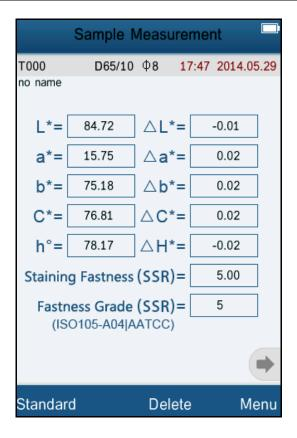
Figure 30 Staining Fastness Measurement
