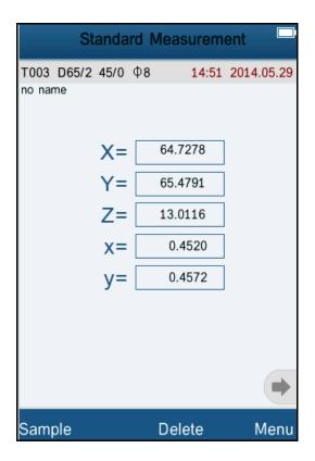
Figure 23 CIE XYZ Standard Measurement
