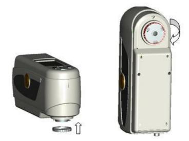
Note: After switching the measuring aperture, you have to adjust the settings (see chapter 6.3).
