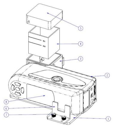
Fill the tank (4) with the medium to be measured and put it into the measuring chamber (3). Make sure the filling level lies between the MIN and the MAX indication of the tank. The tank has two sides with a dull surface. Only touch it on those two sides to prevent measurement errors due to dirt.
