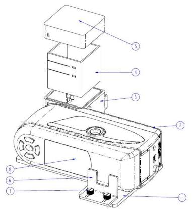
2. Fill the cuvette (4) with the desired medium and put it into the measuring chamber (3). The cuvette has two matte surfaces at the sides. Only touch it on those two sides to prevent measurement errors due to dirt. The cuvette is also equipped with a filling level indicator. Make sure the filling level lies between the MIN and the MAX indication of the tank.
