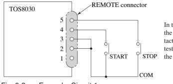
In this example, controlling the START and STOP contacts lets you operate the tester in the same way as from the front panel.
