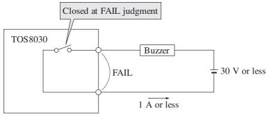
Fig. 7-2 Example: Use of FAIL Signal
