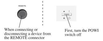
Fig. 6-1 REMOTE Connector and POWER Switch
