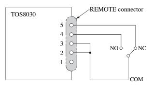
In this example, setting the contact to the NO position invokes a TEST state; returning it to the NC position stops testing.
