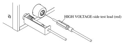
Connecting the HIGH VOLTAGE-side test lead Fig. 3-4
