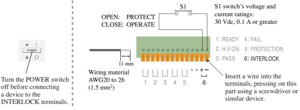
Fig. 6-6 Connecting a Device to the INTERLOCK Terminals
