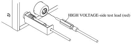
Fig. 3-8 Disconnecting the HIGH VOLTAGE-side Test Lead
