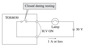
Fig. 7-3 Example: Use of an H.V ON Signal
