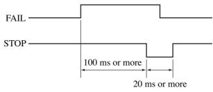
Fig. 6-5 Timing of a STOP Signal
