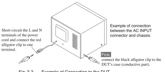
Fig. 3-3 Example of Connection to the DUT
