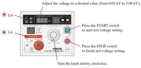
Fig. 5-9 Setting the Test Voltage
