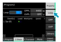
Use the numeric keypad or the rotary knob to enter number of loops.
