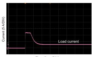
■ Measurement conditions Operation mode: CC Load current: 0 A→12 A DC INPUT terminal voltage: 800 V
