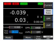
Use the numeric keypad or the rotary knob to enter the slew rate value.
