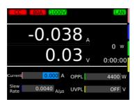
By factory default, the panel settings immediately before the POWER switch is turned off are saved. When you turn the power on, the product starts in the same state as it was in the last time it was turned off. (However, the load setting is always Load Off.)
