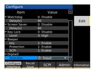
Use the rotary knob to select Input (digital input) or Output (digital output), and then press ENTER.
