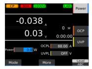
Use the numeric keypad or the rotary knob to enter the power value.
