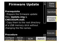
Insert the USB memory device on which the update files have been saved into the USB port on the front panel, and then press Execute.
