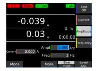
Use the numeric keypad or the rotary knob to enter the sine amplitude (Amplitude). The amplitude is a P-P value with the center value at the load value. This completes the setting.
