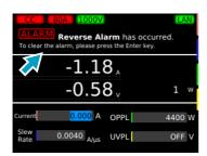
If a reverse voltage of -5 V or higher is applied or a reverse current (approximately -1 % of the rating) flows, a beeping sound is generated and a reverse alarm (reverse-connection detection) appears.
