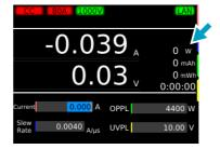
Display example of integrated current, integrated power, and elapsed time
