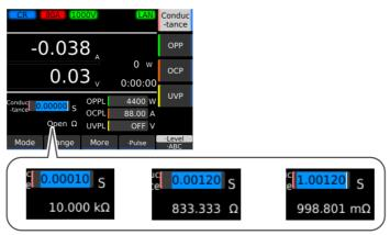
Resistances are displayed with k for kilo or m for milli. Up to three decimal places are displayed.
