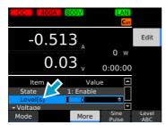
Use the numeric keypad or the rotary knob to enter the value for activating the cutoff, and then press ENTER.
