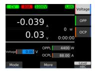
Use the numeric keypad or the rotary knob to enter the voltage value.
