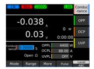
Use the numeric keypad or the rotary knob to enter the conductance value.
